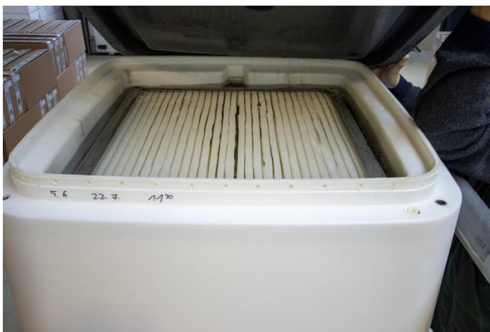
Figure 4: example of a water-PCM-battery module at the top of a buffer with 80 mm isolation (lit. 2).
